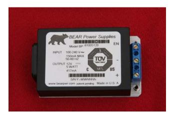
The BEAR power supply survived the level 1and level 2 lighting surge tests and continued to operate properly after each test.
