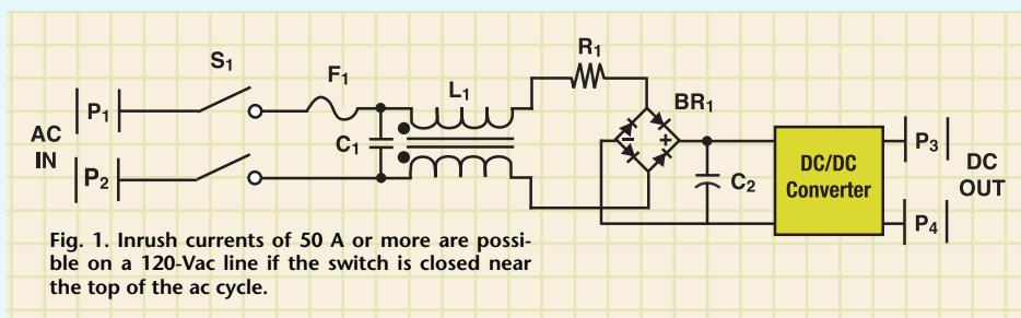
Fig. 1. Inrush currents of 50 A or more are possible on a 120-Vac line if the switch is closed near the top of the ac cycle.
