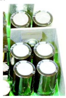
This poorly designed power supply surrounds its storage capacitors with a large heat sink designed to dissipate significant heat. High temps degrade capacitor performance over time, reducing storage capacity and magnifying ripple. Power supplies designed for long life have capacitors sitting away from heat sinks and other high-temperature components.
