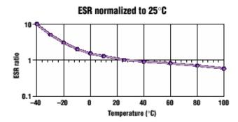
Effective series resistance, or ESR, of capacitors rises as temperature falls. High ESRs reduce storage capacity while boosting ripple in the output of the capacitor. A supply that meets specifications at room temperature may fail to reach them at -20°C.
