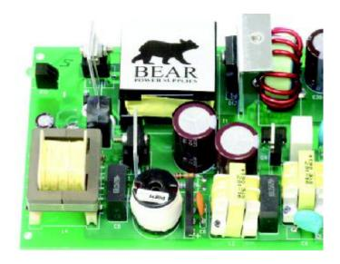
Power supplies designed with openly spaced components operate at lower temperatures than supplies with tightly packed circuit boards. Lower operating temperatures help extend the life of the supply.
