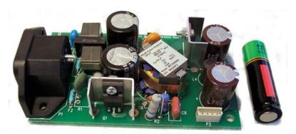
Since this power supply is used in an un-vented plastic enclosure, the specified operating temperature is much higher than the ambient hospital room temperature. (Photo by BEAR Power Supplies)
