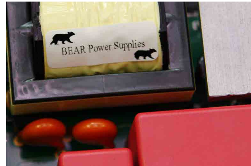
Figure 5: Two small Y-caps (orange) between the primary and secondary help meet EMI specs.
